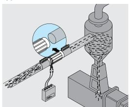
Install a Conveyostat prior to the cyclone in a slitter trim application to neutralize the static charges that cause material to stick to the sides of the exit duct and send false signals to the baler, allowing the material to flow smoothly.
