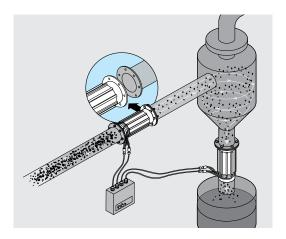
Remove static charges generated on plastics by installing a conveyostat before and after the cyclone to keep the material moving freely.
